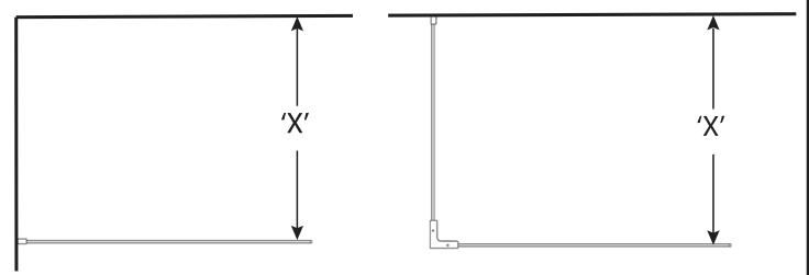
Measure from inside of glass to back wall (X). Remove wall bracket, & with clamping mechanism pushed fully into bar, cut bracing bar at wall end ONLY, to:
