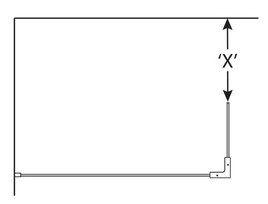
1. Ensure Plumb then measure from end of ÿxed bypass panel to back wall (X). Remove wall bracket from bracing assembly.
