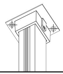
3. Apply continuous bead of silicone sealant in glazing channel of post from base to top of glass height (1980mm)
