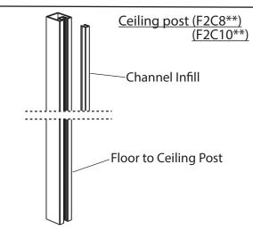
1. Measure from base of panel to ceiling (X) and cut Floor to Ceiling post to X-5mm.
